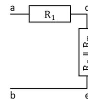
$$V_{de} = \frac{(R_2 \parallel R_T)}{(R_2 \parallel R_T) + R_1} V_{ab}$$
