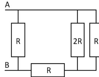
$$\begin{aligned} R_{eq} &= R \parallel (R + (2R \parallel R)) \\ &= R \parallel \left( R + \frac{2R}{3} \right) \\ &= R \parallel \frac{5R}{3} \\ &= \boxed{\frac{5R}{8}} \end{aligned}$$
